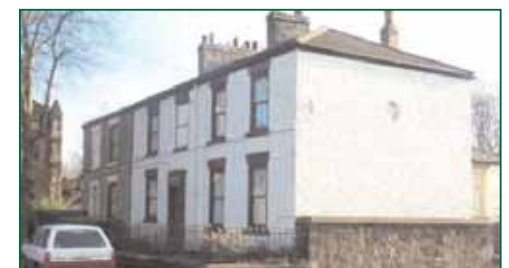
An example of a traditional style dwelling, found throughout the coalfield area, with slate roof, sash windows and simple door surround.
