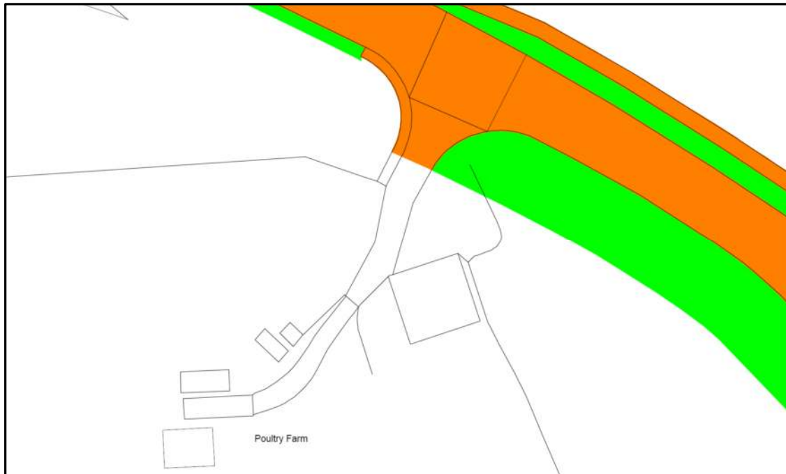
Figure 2: Location of Adopted Highway (Orange) and Adopted Highway Verge (Green) in relation to site access and existing bellmouth/footpath access.
