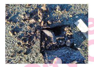
The floor - felt roof (Bitumen) (Area: 2 Roof 2) does not contain asbestos.
