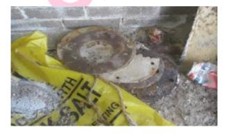
The redundant flange gaskets to floor in Gas Meter cupboard do not contain asbestos.
