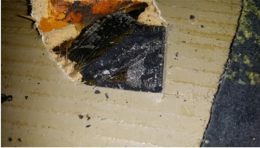
The covering below two layers of floor covering in Rm 021/Corridor does not contain asbestos.
